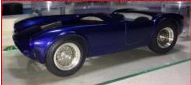
Body resting on the chassis with wheels tentatively set in place.
