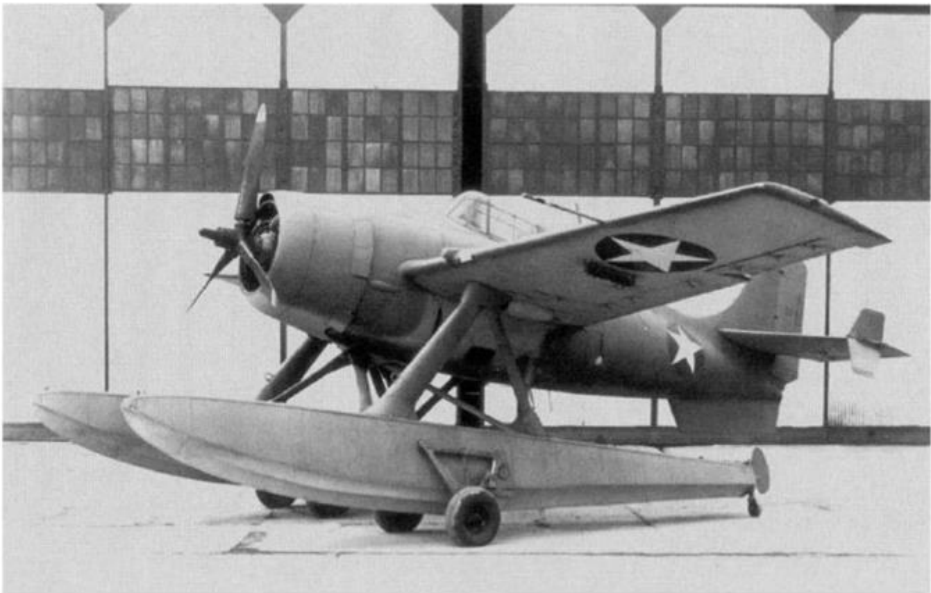
Another view of the real thing that highlights the two beaching dollies
